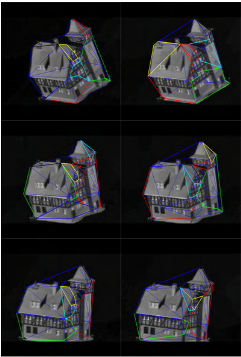
Fig. 6. Graph partition on Delaunay triangulations
